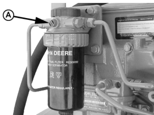
Final fuel filter bleed screw
