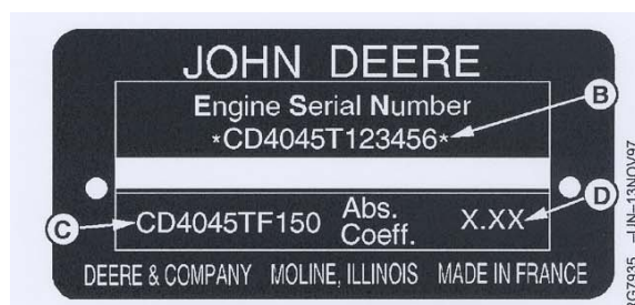
Figure 1.7: Example of generating set identification plate
