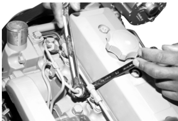
Bleed fuel system at fuel injection nozzles
