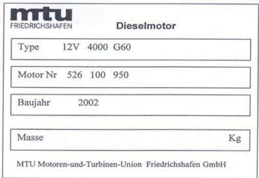
Figure 1.3: Example of generating set identification plate
