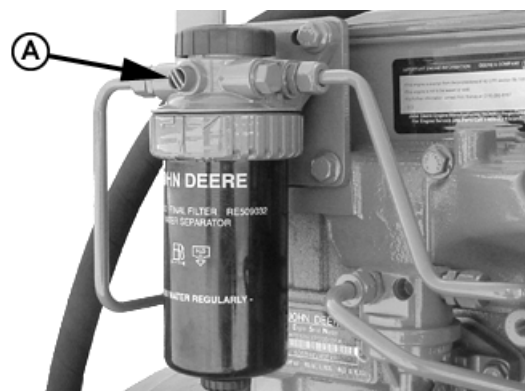
Final fuel filter bleed screw
